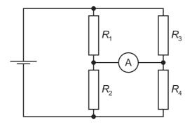
The four resistors have different resistances  $R_1$ ,  $R_2$ ,  $R_3$  and  $R_4$ .
