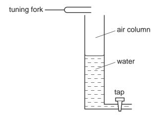
The tube is filled and then water is allowed to run out of it. The first two stationary waves occur when the air column lengths are 0.14 m and 0.42 m.
